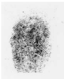
FIG. 2—Blue-colored fingerprint developed with genipin on copier paper and recorded under white light illumination.
